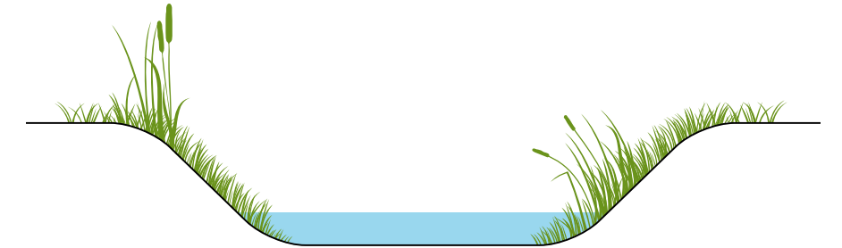
W3 for approx. 20m lengths, with distance between aquatic margin centres approx. 100m – 200m
